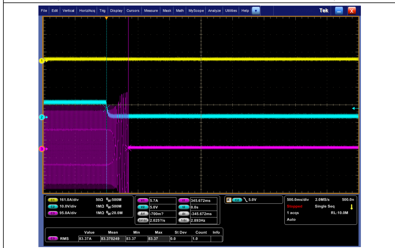
Graph of disconnection at P_{AC} 0% and Q_{AC} 0% reactive load and 100% nominal power
