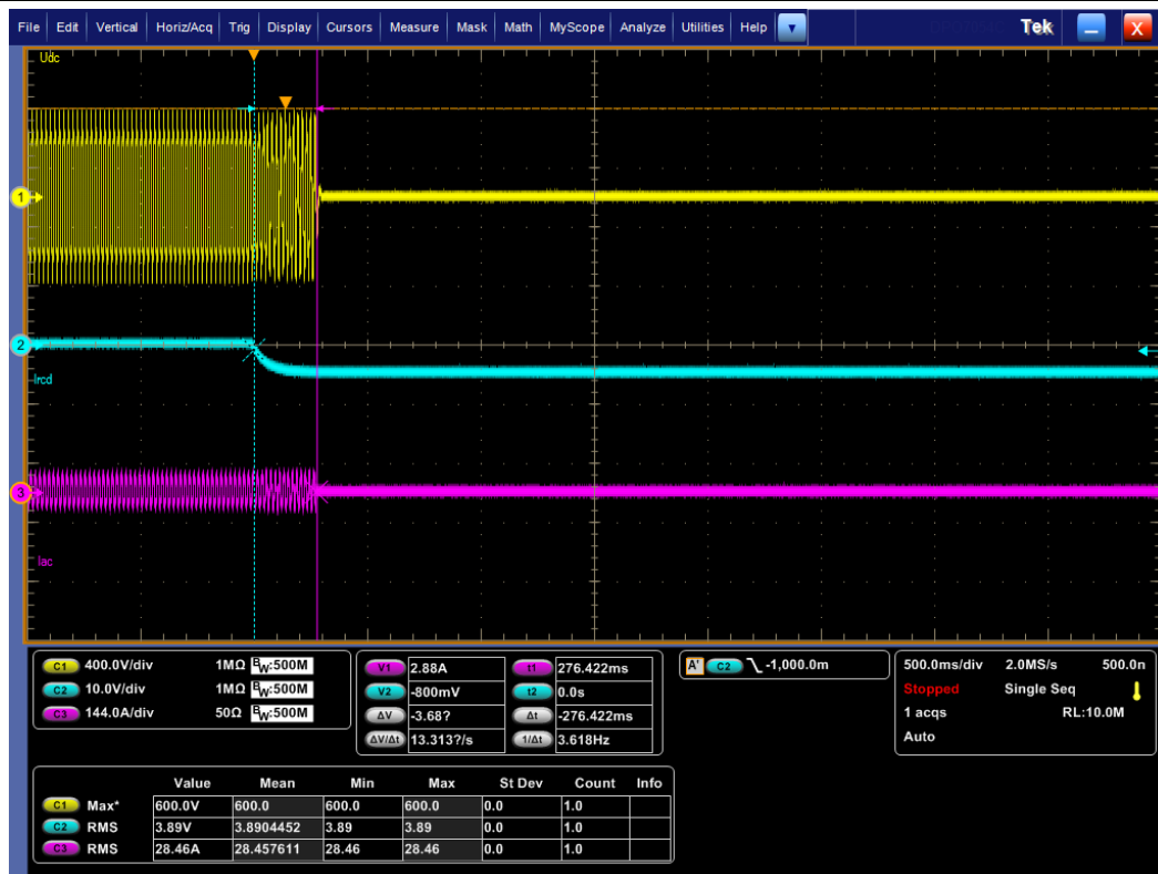
Graph of disconnection at P_{AC} 0% and Q_{AC} -5% reactive load and 33% nominal power
