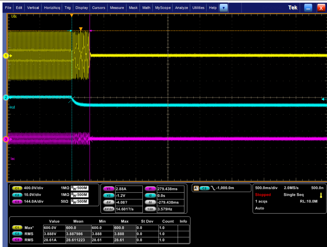
Graph of disconnection at P_{AC} 0% and Q_{AC} -5% reactive load and 33% nominal power
